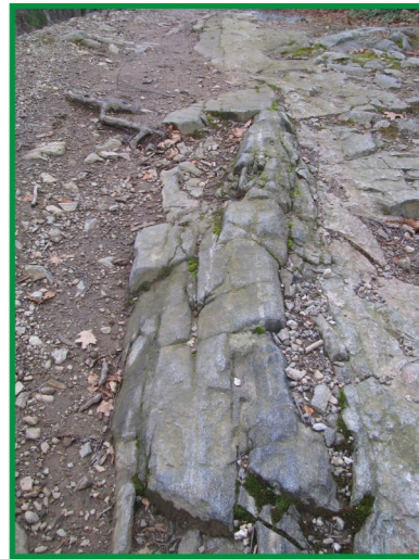
Vertical bedrock fractures in unpaved roadway immediately southeast of Mountain Lake Orientation: N31°E to N38°E
