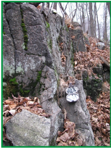
Vertical fractures located near the southwest end of Mountain Lake. Orientation: N32°E
